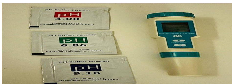
Figure 2. Calibration and use of the digital pH meter for immediate measurement of unstimulated whole SpH using standard buffer solutions (pH 4.00, 6.86, and 9.18).
