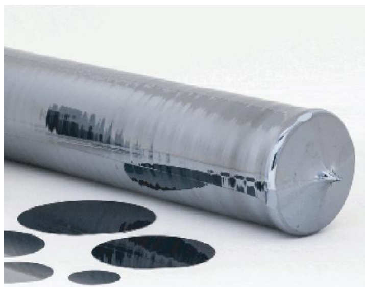
Figure 3: A silicon ingot with thin silicon wafer sliced off.
